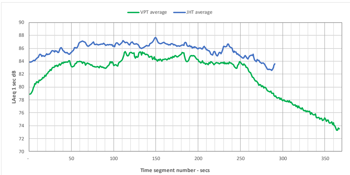
Figure 9 Broadband noise levels along the two tunnels.
